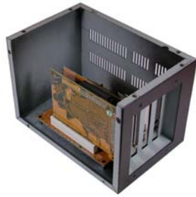
Installing PCI Add-in cards inside the Expansion Box
